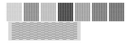
5. The utility prints and checks up to five times. If some print head nozzles are still clogged, it displays an on-screen message telling you to manually clean the print head. Follow the instructions on page 79 to clean the print head, if necessary.
